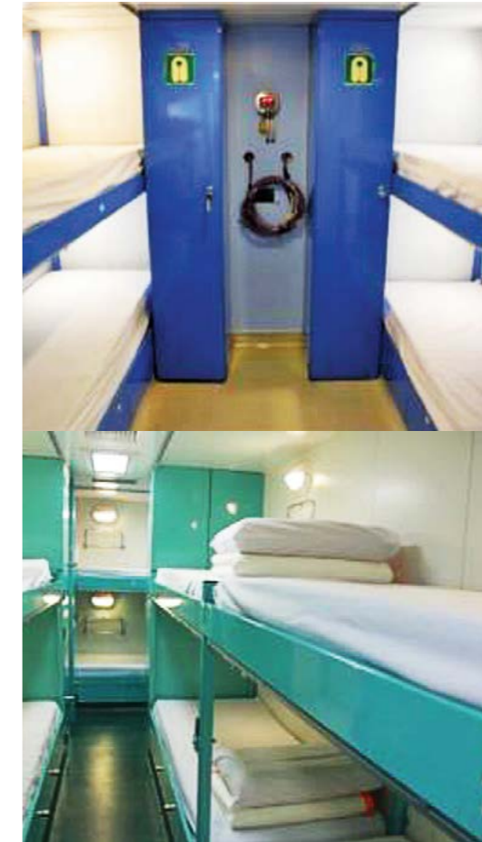
Shipboard isolation (top) and quarantine (below) facilities with separate ventilation air flow circuits on board RSN ships to enable Recover@Sea. Source: MINDEF
